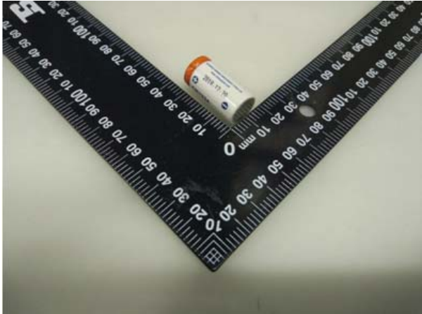
电池/ Battery(CR123A 3,0V 1500mAh)
